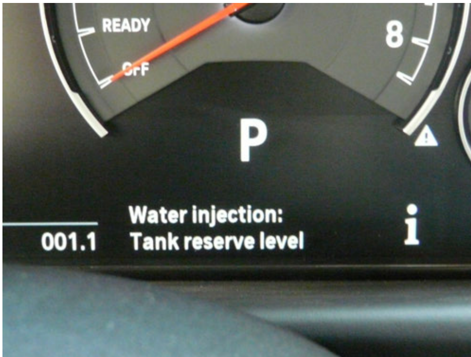
Water injection Tank Reservoir Low Level display in cluster
